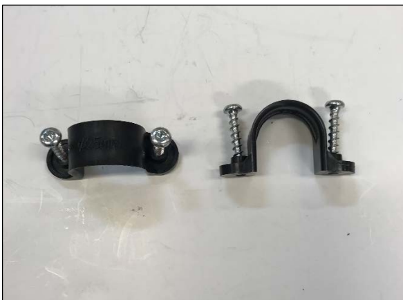
Fig. 3.3: Clamps for conduit pipe (25 mm)
